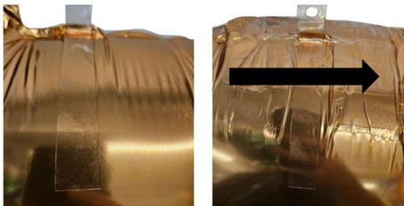
~ 6" of packing tape placed perpendicular to the hang tabs
